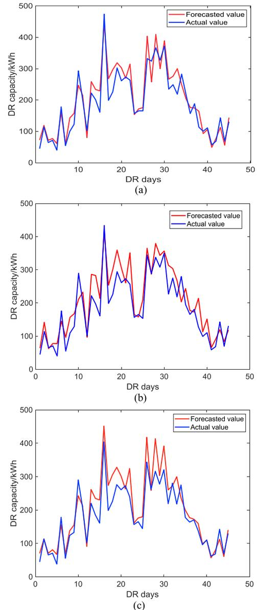
Fig. 6. Forecasting results: Comparison of the forecasted and actual values of the aggregated DR capacity under three different distributions of customers. (a) Distribution 1. (b) Distribution 4. (c) Distribution 7.
