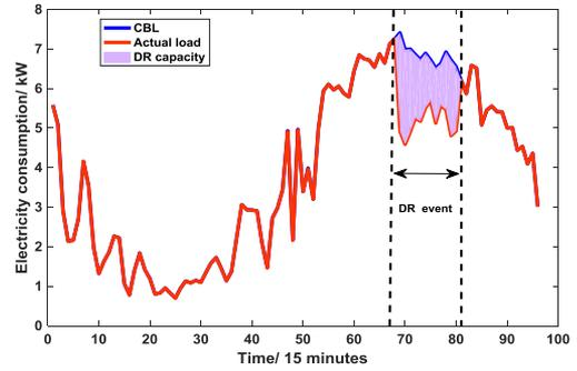
Fig. 2. Schematic diagram of the DR capacity.
