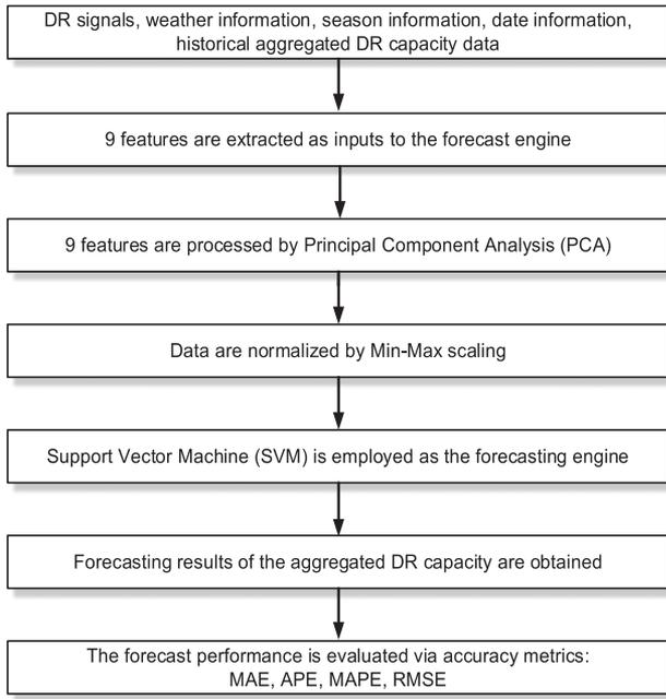
Fig. 5. Overall forecast structure.
