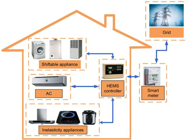
Fig. 4. Schematic diagram of the smart household.
