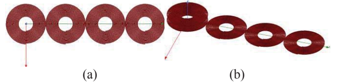
Fig. 7. ANSYS Simulation of coils with distance between transmitters 0 cm: (a) top view, (b) 3D view
