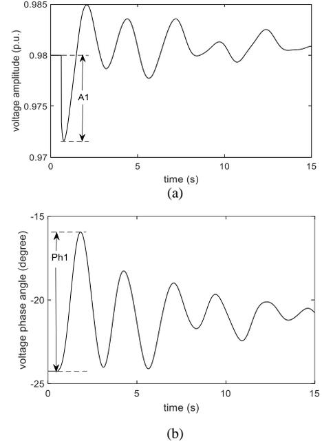
Figure 3. First peak in (a) amplitude and (b) phase angle of a voltage phasor
