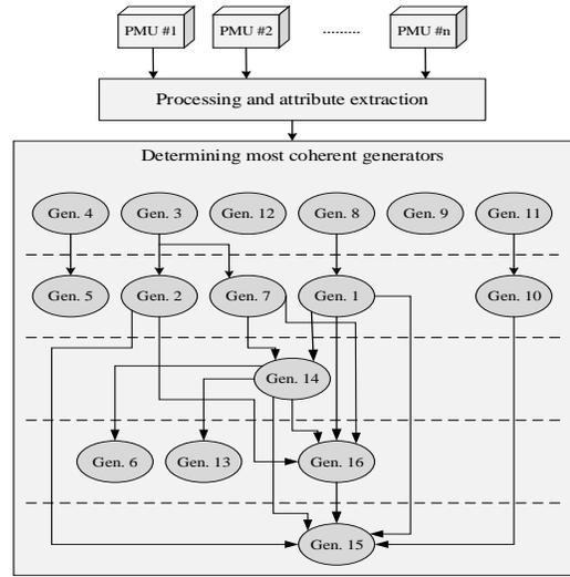
Figure 5. Hierarchical scheme for most coherent generators determination
