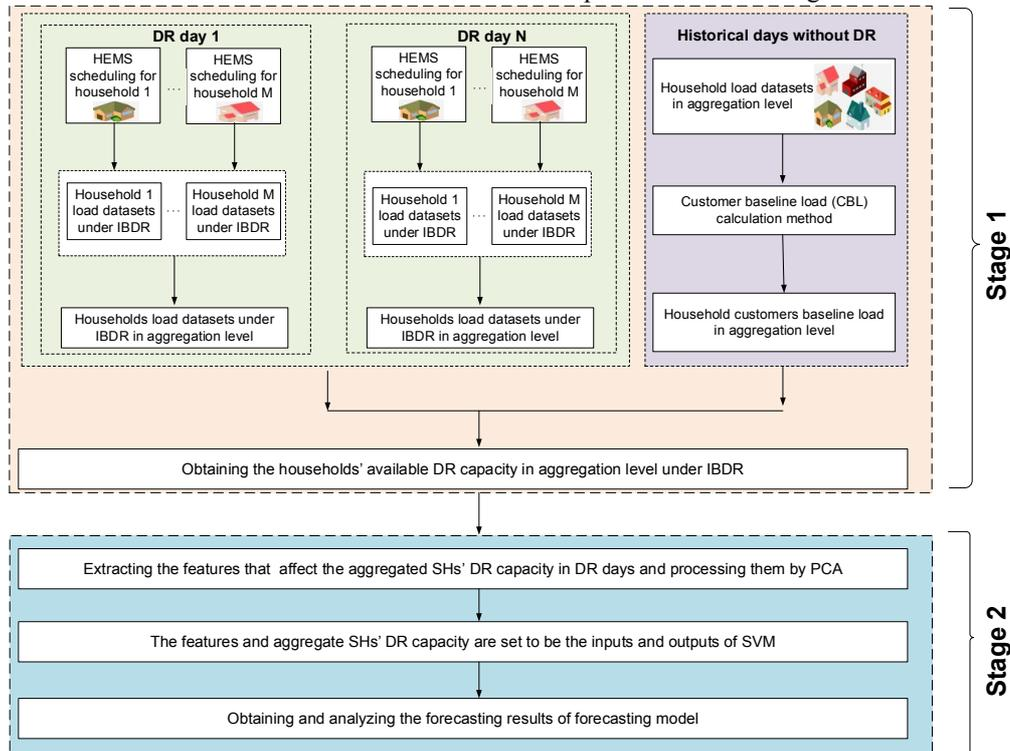
Fig. 3. Architecture of the proposed framework for aggregated DR capacity forecast
