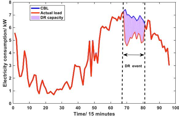
Fig. 2. Schematic diagram of the DR capacity
