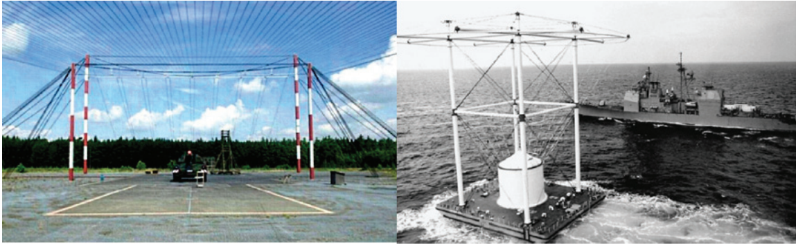
Figure 2.5: Guided-wave HEMP Simulator(left) And Dipole Simulator(Right)
